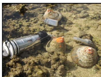
Figure 3. Trocas equipped with accelerometer sensors
